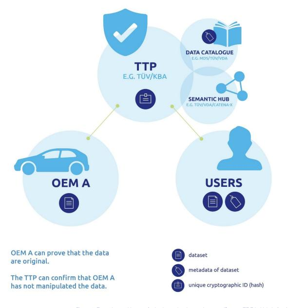
Figure 1: Exemplary architecture for implementing the requirements (Source: ZF Friedrichshafen AG) TTP: Trusted third party TÜV: Technischer Überwachungsverein or Technical Inspection Association KBA: Kraftfahrt-Bundesamt or Federal Motor Transport Authority MDS: Mobility Data Space VDA: Verband der Automobilindustrie e. V.or German Association of the Automotive Industry
